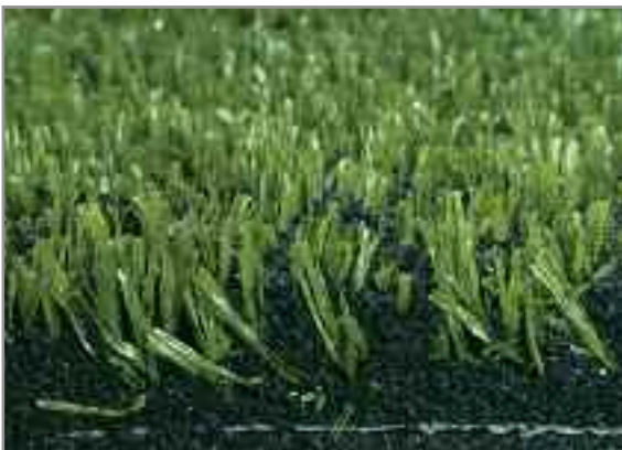
Cross-section view of turf with (optional) rubber infill.
